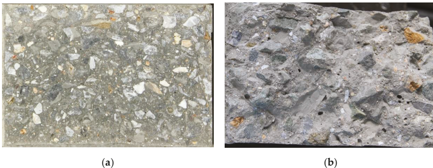
Figure 7. The fracture surface of concrete at different temperatures: (a) at 5 °C; (b) at 60 °C.
