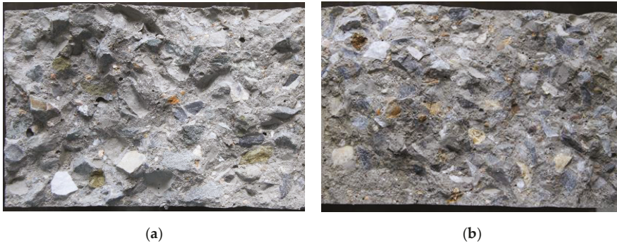
Figure 6. The fracture surface of concrete at different ages: (a) at 3 d; (b) at 60 d.
