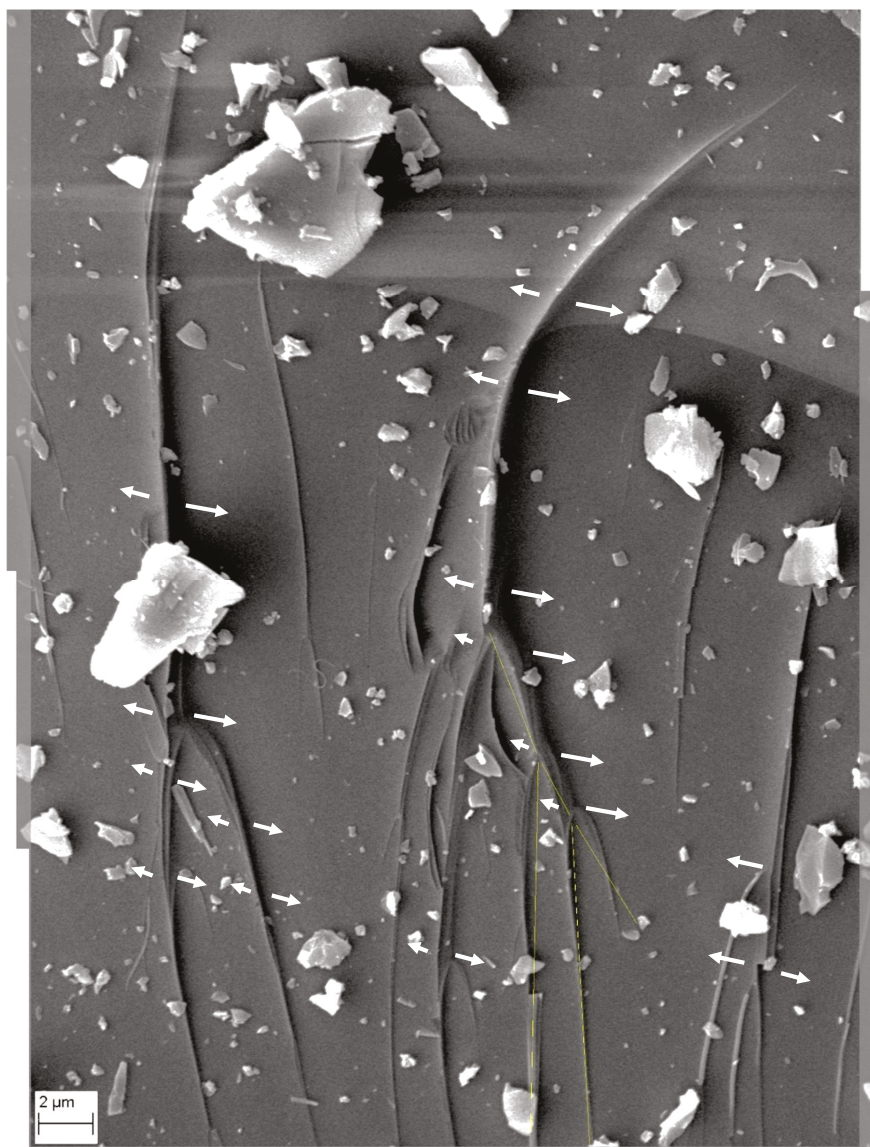
Figure 6. Fractures on the surface of a quartz granule subjected to 100 MPa; the bifurcations show angles of about 27^\circ (taken from the work of Martinelli et al. [5]).
