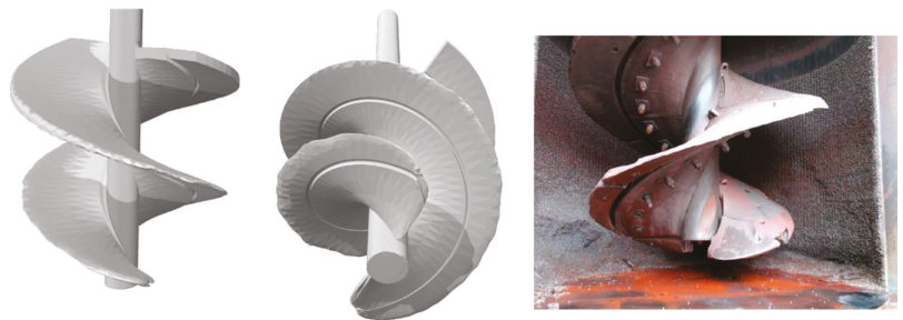
Figure 20. Comparison between 3D worn screw after DEM simulation and industrial worn liner.
