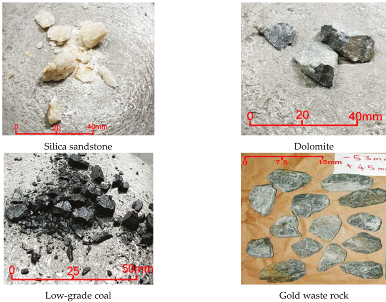
Figure 5. Display of the samples of material used in the drop weight tests.
