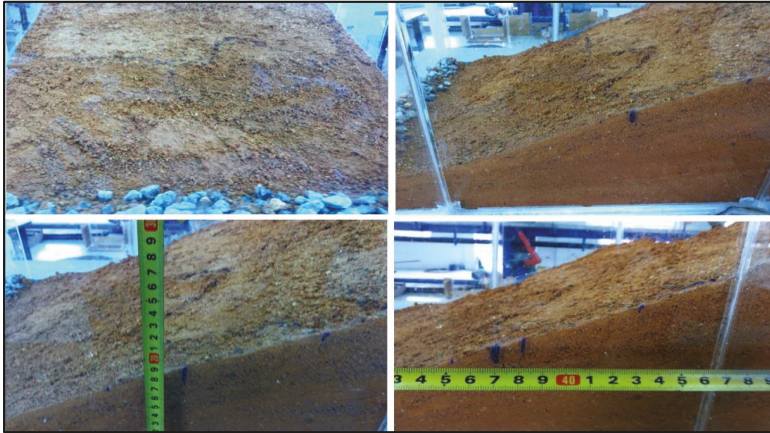
Figure 4. Seepage line touches the downstream slope of the model with toe drain.
