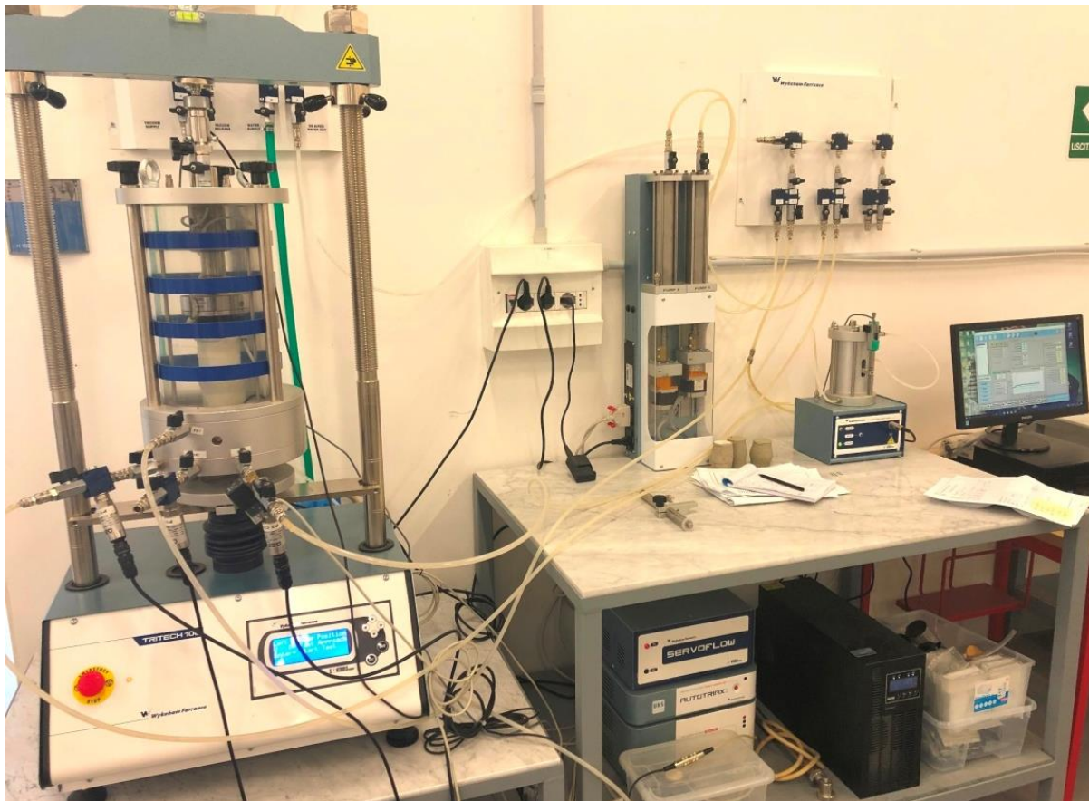
Figure 12. Triaxial machine for unsaturated soil in the Geotechnical Laboratory of the University of Enna “Kore”.
