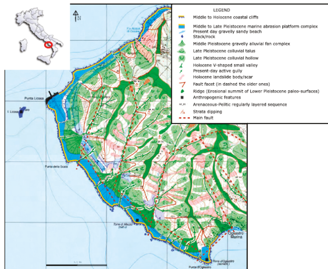
Figure 12. Geomorphological map of Licosa Cape made with the GmIS_UniSa procedure [40].
