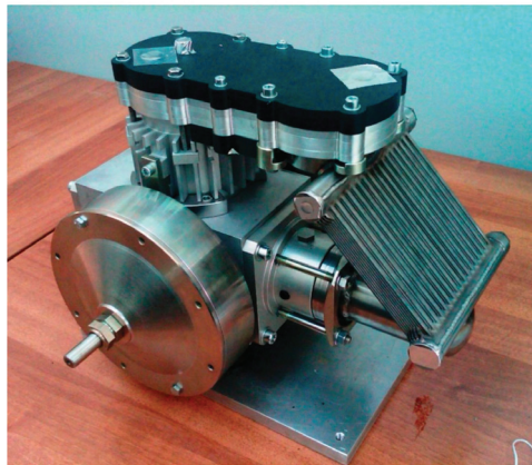
Figure 12. Manufactured Stirling engine with an additional heat exchanger attached for operation with a solid fuel boiler [79,80].
