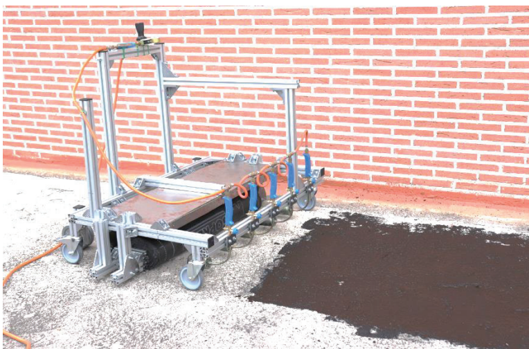
Figure 14. Prototype and surface ready for asphalt roofing.
