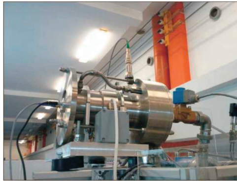
Figure 23. Radial, single-stage steam microturbine installed on the Institute of Fluid Flow Machinery test stand [148].
