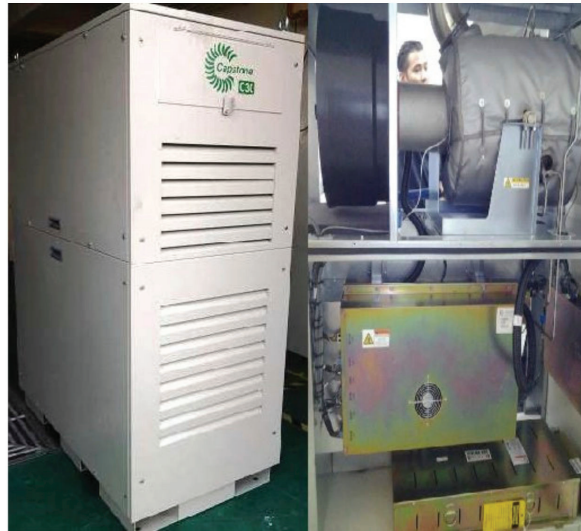
Figure 20. View of the Capstone 30 kW gas turbine [134].
