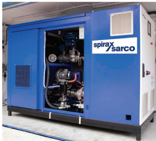
Figure 24. View of the Spirax Sarco steam microturbine [153].
