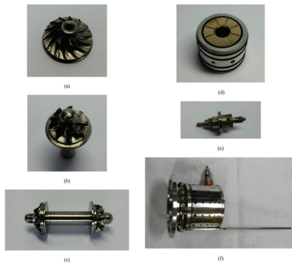
Figure 19. Elements of the first integrated test rig: (a) compressor, (b) turbine, (c) rotor shaft with compressor and turbine, (d) radial-thrust integral static air bearing, (e) graphite hot-bulb igniter and (f) annular-type combustor with 12 nozzles [125].
