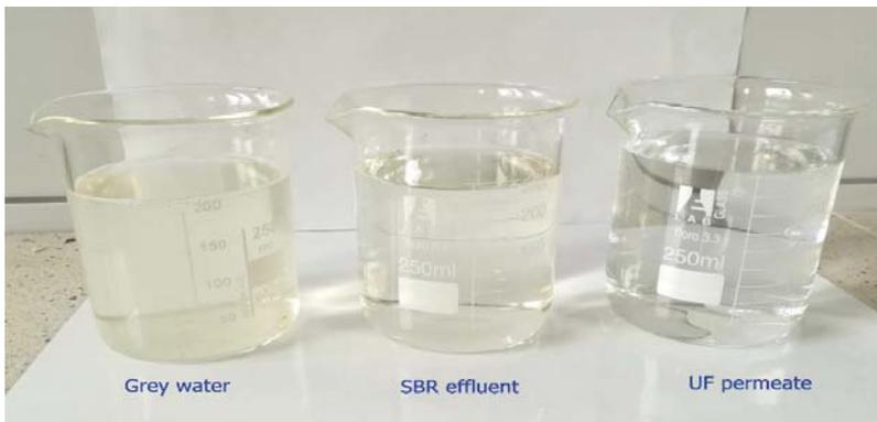
**Figure 5.** Changes in the color and the turbidity of grey water under treatment with SBR followed by ultrafiltration.
