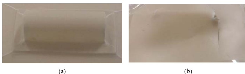
Figure 1. Thermoformed samples containing 60 wt.% starch (a) and 70 wt.% starch (b).
