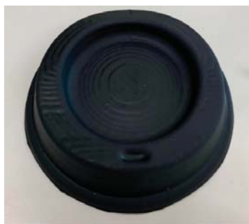
Figure 4. Thermoformed coffee lid made with 10 wt.% biochar from spent coffee grounds.
