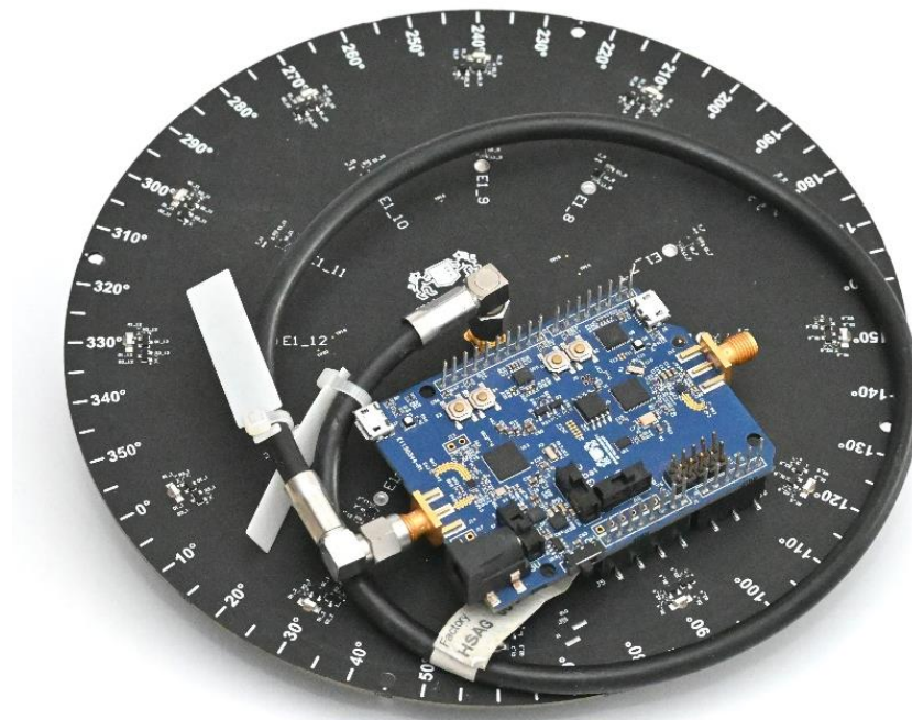
Figure 6. The ESPAR antenna connected to the custom-made nRF52840 wireless sensor network (WSN) board via Arduino Shield header pins. The WSN board's radio frequency (RF) signal output is connected to the ESPAR antenna's center element via a black SMA cable.
