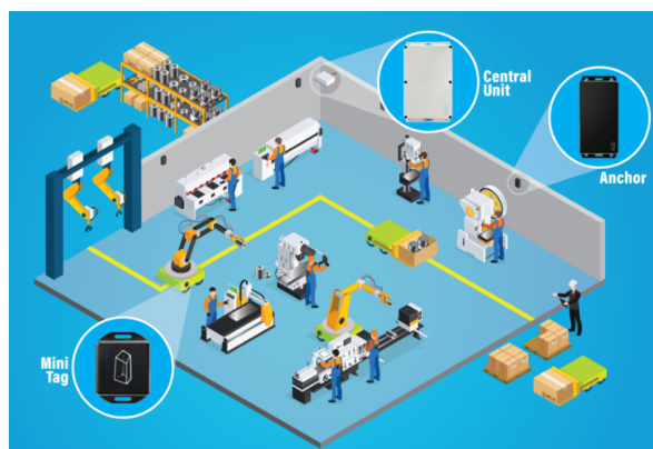
Figure 8. The infrastructure of the Sunstone-RTLS. Every central unit (CU) has eight anchors (which collect data from tags), and the CUs can be connected to create a cascade installation.
