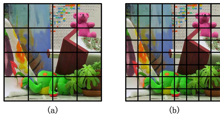
Figure 5. Schematic diagram of meshing: (a) image divided by 4 \times 4 sub-regions, (b) image divided by 8 \times 8 sub-regions.
