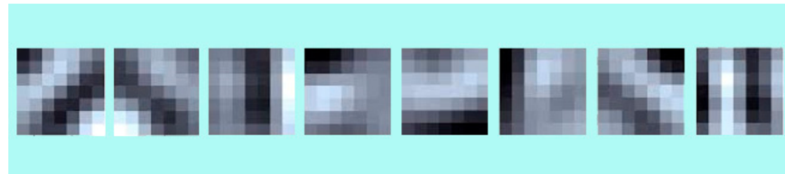
Figure 2. Examples of 7 \times 7 BSIF filter banks learned from natural pictures.
