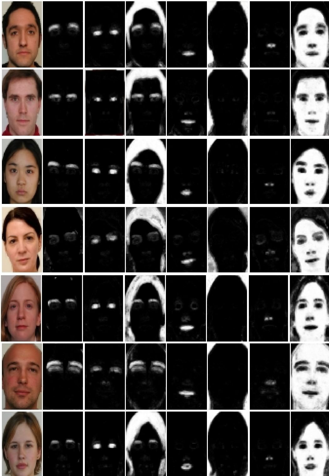
Figure 5. Example face images from FASSEG [29] database, probability maps in the order such that: column 1 shows: original images, 2: eyebrow, 3: eyes, 4: hair, 5: mouth, 6: back, 7: nose, and 8: skin class.
