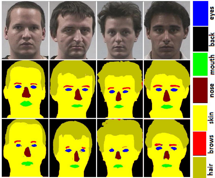
Figure 1. Face parsing results for FASSEG [29] frontal images. First row show: original images, second row: ground truth, and third row: face parsing results.
