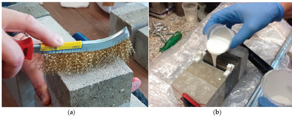
Figure 4. Preparation of a specimen for tests: (a) cleaning the surface and (b) pouring the resin into the expansion joint.
