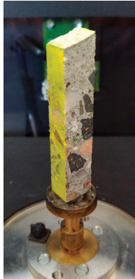
Figure 17. The sample attached to the holder and mounted in the chamber of X-ray scanner.
