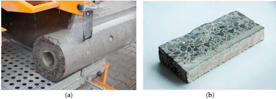
Figure 2. Preparation of test samples: (a) cutting off the top of the pole; (b) a slice of concrete intended for laboratory testing.
