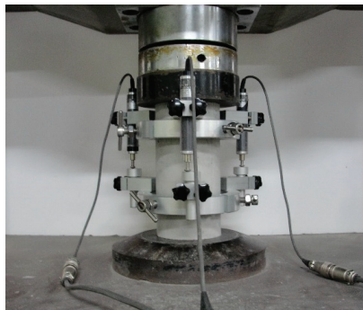
Figure 1. Experimental setup for determining static elastic modulus and compressive strength of concrete specimens.
