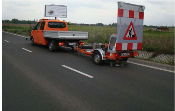
Figure 12. View of the FWD device during the test.
