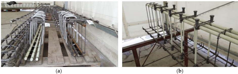
Figure 2. Reinforcement details of test specimens based on example beams: (a) B-1 and B-2; (b) B-3.
