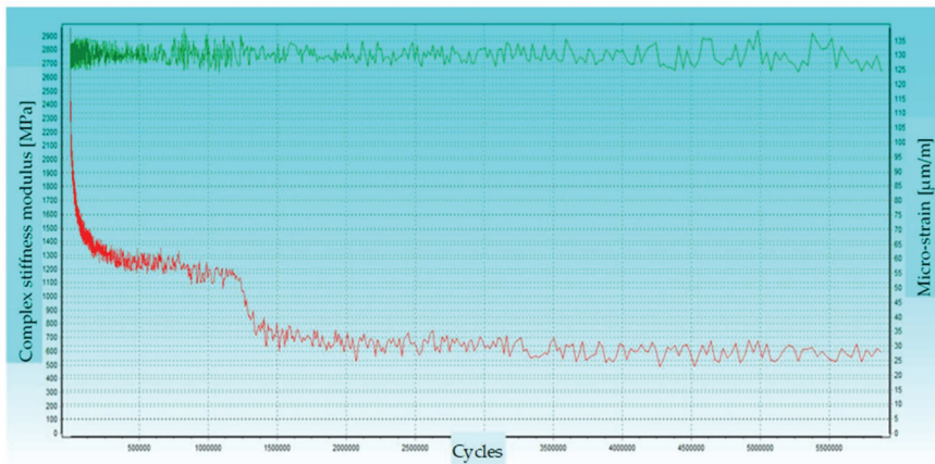
Figure 6. The course of the FAC mixture fatigue test at standard load.
