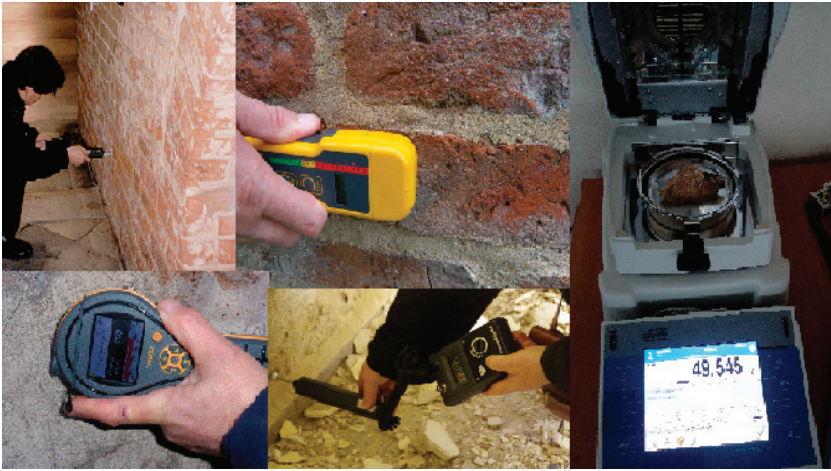
Figure 2. Testing areas and measurement techniques (nondestructive and destructive).
