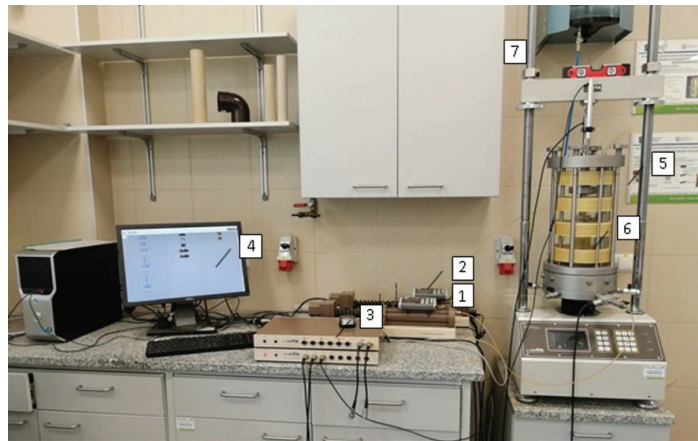
Figure 3. Set-up of dynamic testing system at Water Centre in Warsaw University of Life Sciences: (1) back pressure controller, (2) cell pressure controller, (3) data logger, (4) PC and control software, (5) frame, (6) cell, (7) water tank.
