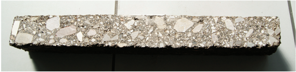
Figure 6. Sample for testing with the four-point bending test on prismatic materials (4PB-PR) method.
