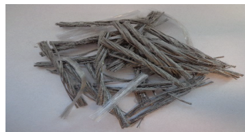
Figure 1. Synthetic structural polypropylene fibres l = 54 \text{ mm} .
