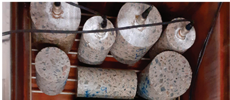
Figure 1. Arrangement of the test specimens with AE sensors in the KD 20 equipment during F-T cycles.
