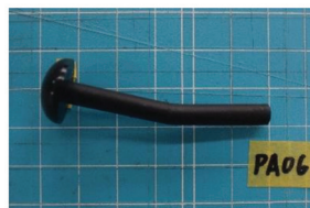
Figure 10. Failure mode of FRTP rivet under bending.
