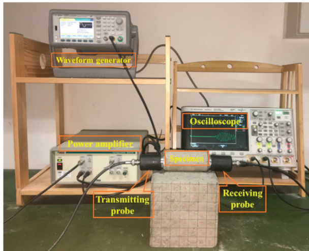
Figure 4. Ultrasonic testing setup.
