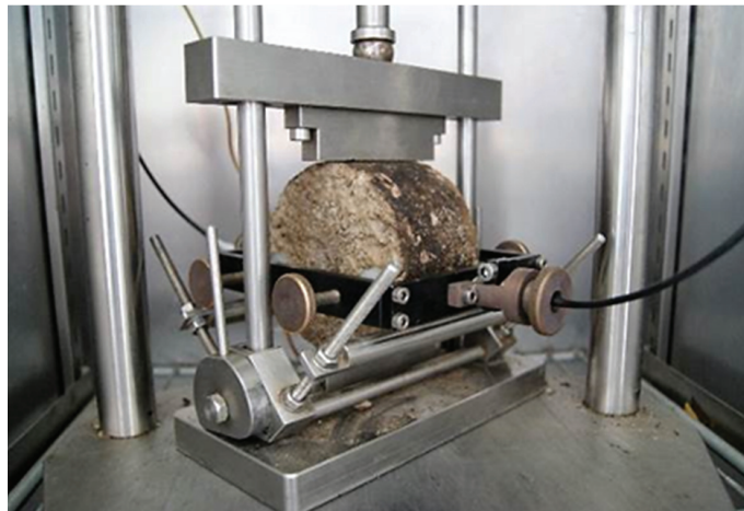
Figure 5. Scheme of the indirect tension test on cylindrical specimens (IT-CY) study.
