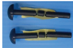
Figure 7. Failure mode of FRTP rivet under shear loading.
