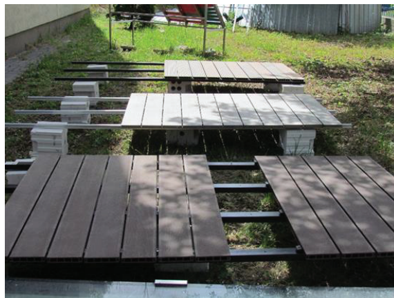
Figure 2. The view of wood-plastic decking profiles during exposure in natural conditions.
