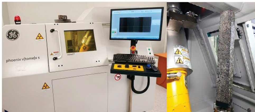
Figure 15. Computed tomography and mounted specimen.
