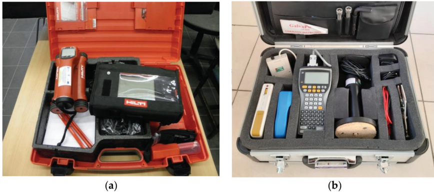
Figure 4. Measuring devices: (a) PS 200 Hilti scanner, (b) GP-5000 GalvaPulse™ kit.
