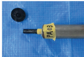
Figure 4. Failure mode of FRTP rivet under tensile loading.
