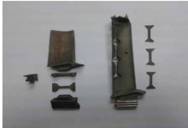
Figure 7. View of specimens cut out (using the electro-discharge method) of a material of the LPT blade and view of specimens for static tensile testing cut out of the material of the HPT blade and LPT blade.
