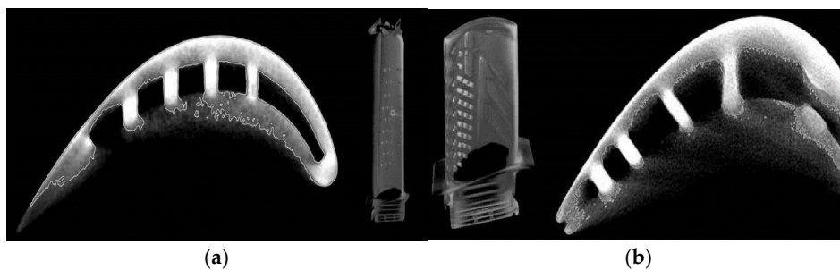
Figure 6. The shape of the LPT blade (a) and the HPT blade (b), with visible cooling channels, obtained by the computer-based micro-tomography CT.
