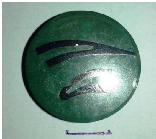
Figure 8. Metallographic specimen of the material of the LPT blade.
