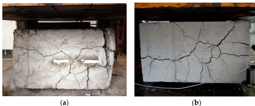
Figure 15. Comparison of failure modes for specimens with different concrete strengths (a) C20 L1 H3 S2; (b) C30 L2 H3 S2.
