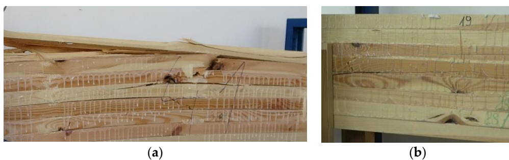
Figure 7. Beam failure images: (a) GL24c—MOR(MOR 12% )—48.5(43.4) N/mm 2 —the strongest in the group, (b) GL28c—MOR(MOR 12% )—30.4(25.8) N/mm 2 —the weakest in the group.
