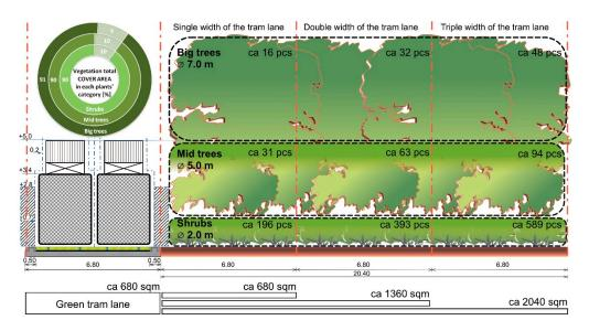
**Figure 19.** Model—Version 1: Land development along the tram route (one-sided intake)—a compact insulating green belt (regular triangular spacing, approx. 90% of the land area coverage). On the left: green tram route cross-section with dimensions—the pictogram after [66]. Compiled by J. Łukaszkiewicz.
