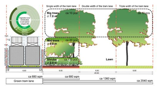
**Figure 21.** Model—Version 3: The linear park. Land development along the tram route with non-regular open forms of high and low greenery, providing for possible recreational use; the required width of the linear park must be at least 3x Tr. On the left: green tram route cross-section with dimensions—the pictogram after [66]. Compiled by J. Łukaszkiewicz.
