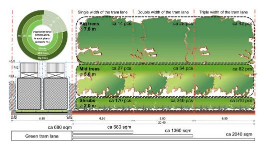
**Figure 20.** Model—Version 2: Land development along the tram route (one-sided intake)—a medium-dense insulating green belt (regular triangular spacing, approx. 80% of the land area coverage). On the left: green tram route cross-section with dimensions—the pictogram after [66]. Compiled by J. Łukaszkiewicz.
