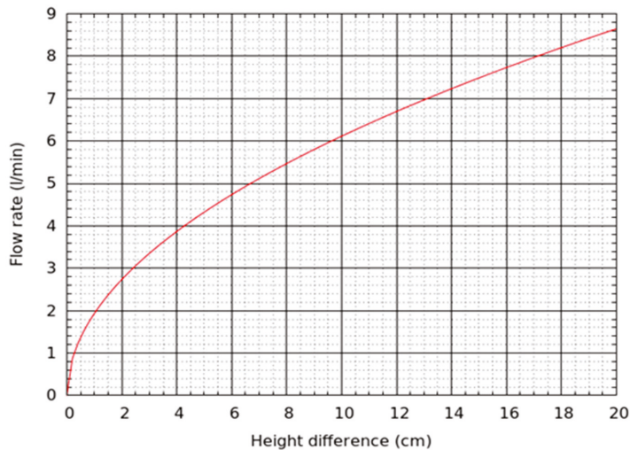
Figure 1. Calibration chart for an orifice plate provided to students.
