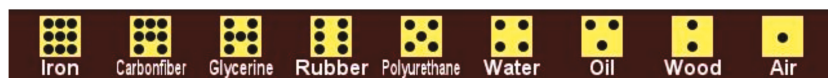
Figure 2. The visual “dots-in-a-box” representation of the density of several materials, reprinted by permission from Springer Nature Customer Service Centre GmbH: Springer, Iterative design of Teaching-Learning Sequences, by D. Psillos and P. Kariotoglou, 2016 and by permission from [20], http://earthlab.uoi.gr/tel/index.php/themeslearn (accessed on 20 March 2021).
