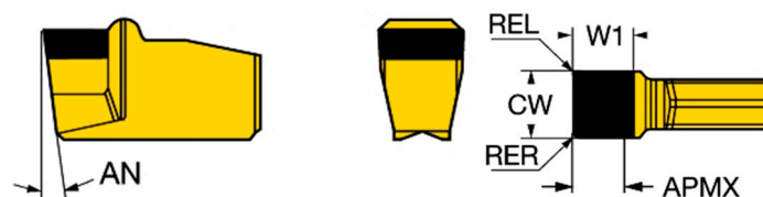
Figure 2. T-Max ® Q-Cut insert for grooving (N151.2-600-50E-G CB20) [11].
