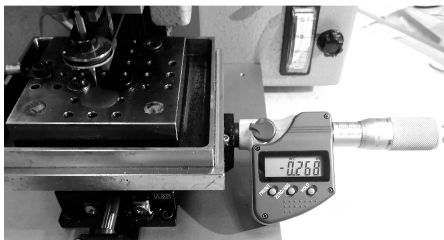
Figure 7. X direction manual control by digital micrometer head.
