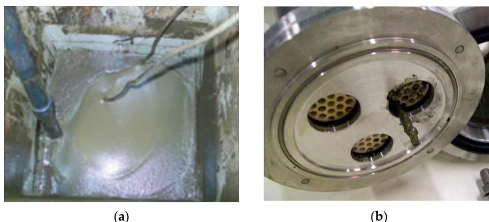
Figure 4. (a) OMW3-SG viscous concentrate after VCR = 2.1. (b) Removal of OMW3-SG muddy concentrate from the membrane channel with a metallic probe.
