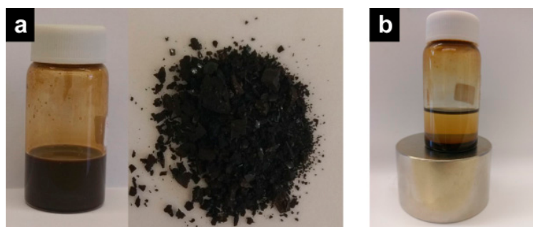
Figure 9. (a) MNPs-IL- \text{C}_4 @PU NCs as suspension and powder and (b) a magnetic separation of MNPs-IL- \text{C}_4 @PU NCs.
