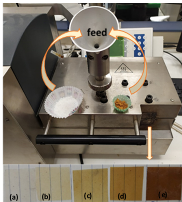
Figure 1. Scheme with the extrusion process used for the preparation of Poly(L-Lactic Acid) (PLLA)/chitosan (CS) and PLLA/CS/BO composites films: (a) “blank” PLLA, (b) PLLA/CS/BO5, (c) PLLA/CS/BO10, (d) PLLA/CS/BO20, and (e) PLLA/CS/BO30.
