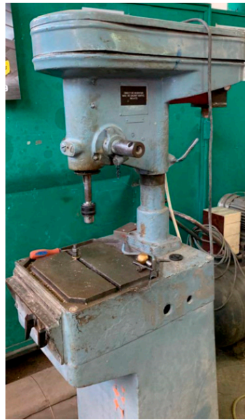
Figure 3. G13 drilling machine used for Friction Riveting.
