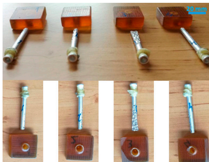
Figure 6. Tested specimens displaying full rivet pullout failure.
