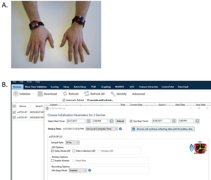
Figure 4. (A): Photo of a participant wearing the Actigraph wGT3X-BT devices on each wrist. (B): A screen shot of the ActiLife software interface used to interact with the wearable device. The software provides options to change various recording parameters (start and stop times, sampling rate, etc.) prior to recording/collecting data.
