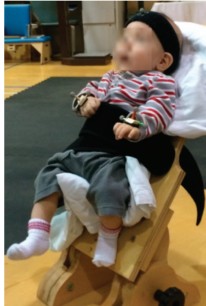
Figure 1. Infant seated in the custom chair and wearing retroreflective markers for 3D motion capture.
