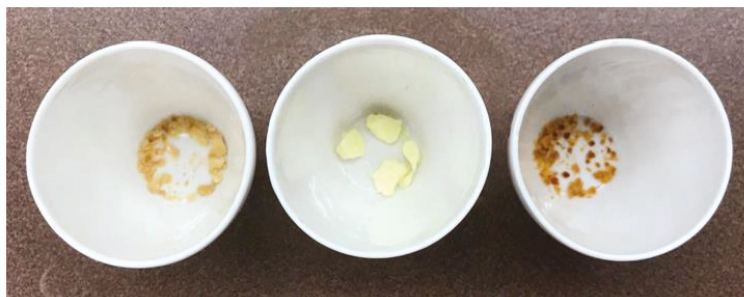
Figure 1. PGE salts from left (Pd, Pt, and Rh) produced by reacting PGE metal powder with potassium bisulfate in a muffle furnace at 550 °C for 3 h.
