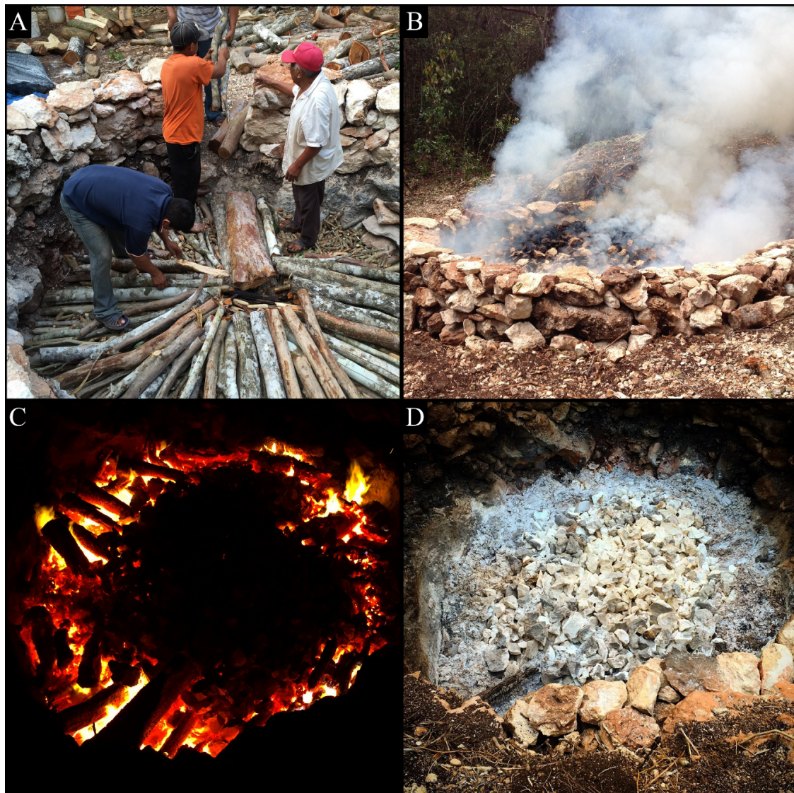
Figure 7. The burnt lime production experiment: (A) the team arranging the fuel for the burn; (B) the kiln heating up soon after being ignited; (C) the fuel burns for a total of 20 h, through the night; (D) by morning, the limestone has been converted to burnt lime [image D adapted from [32]].
