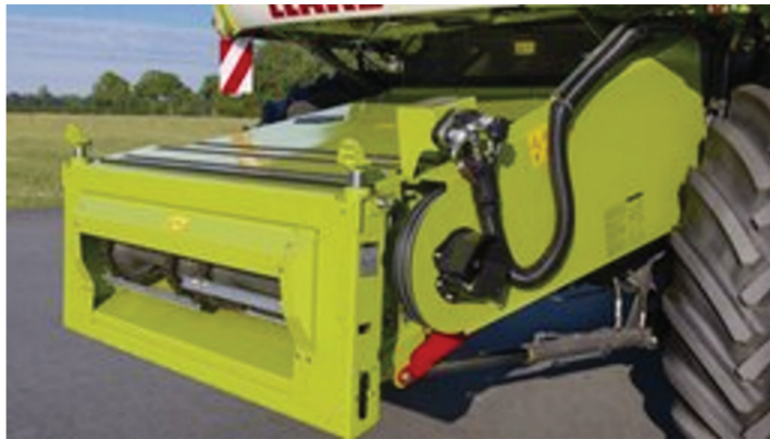
Figure 2. Feeding house attached to the combine harvester body and ready to be attached with a cutting head.
