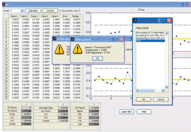
Figure 19. Pattern recognition in X-bar chart by NN.
