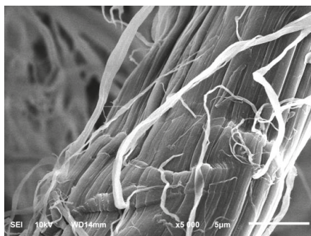
Figure 4. SEM image of aramid fiber after surface treatment with acetic anhydride for 1 h.
