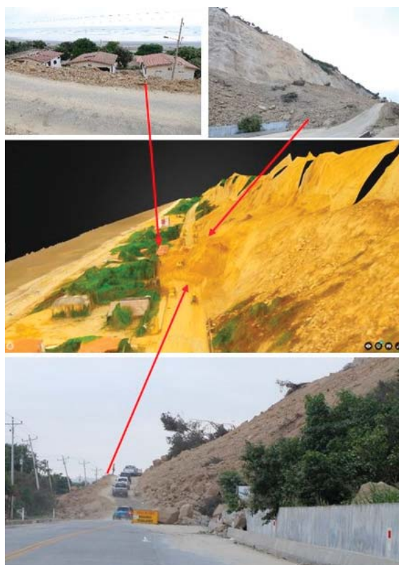
Figure 5. Example of disrupted landslide at Briceño: rock fall and debris displacement, fractured slopes, completely destroyed road, house damaged by landslide, volume ca 10.000 m 3 (VIII ESI-07 ); courtesy of drone imagery by Global Medic and Servicio Nacional de Gestión de Riesgo y Emergencias de Ecuador; locations on Figure 2.
