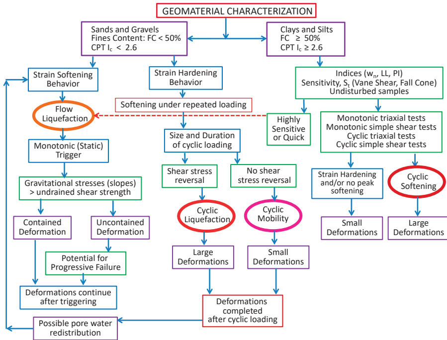
Figure 2. Flow chart showing different types of soil liquefaction: flow liquefaction, cyclic liquefaction, cyclic mobility, and cyclic softening (modified from References [41,42]).
