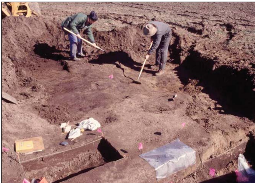
Figure 13. Paleoseismic investigation at an archeological site in the New Madrid seismic zone [130]. The contact between the plow zone and the underlying sand blow is examined for features, such as cultural pits and tree-root casts, that may help to constrain the minimum age of the sand blow. Photograph by M. Tuttle.
