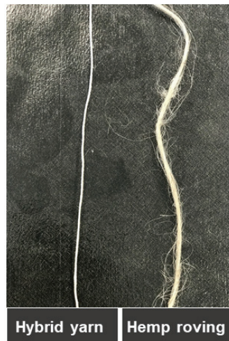
Figure 4. The visual aspect of a hybrid yarn and a hemp roving.
