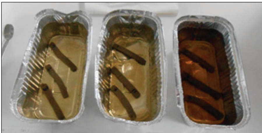
Figure 7. Macroscopical image illustrating the change of the visual of the SPC injection-molded piece-water system upon increasing the solid-liquid contact time (from left to right, 1, 3, and 6 h).
