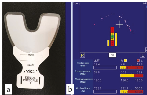
Figure 2. Occlusal force measurement system: (a) pressure-sensitive sheet (Dental Prescale II); (b) image of occlusal condition using software (bite force analyzer).
