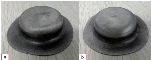
Figure 13. Hot stamping parts of experimentally stamped ZK60 magnesium alloy: (a) Obtained part at the parameters of compromise solutions 1; (b) Obtained part at the parameters of compromise solutions 2.
