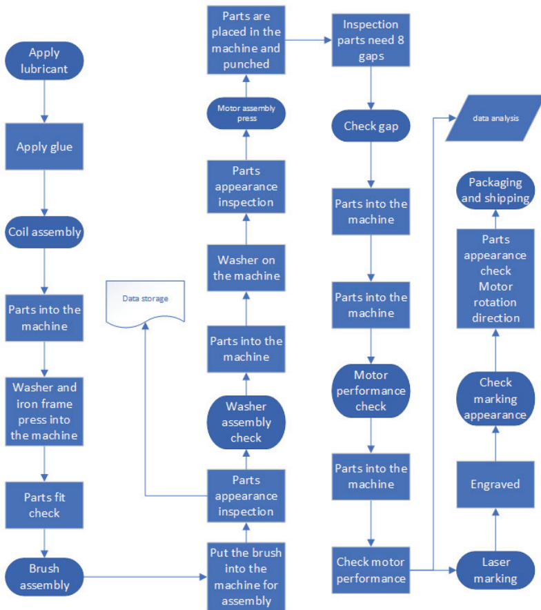
Figure 6. Motor assembly intelligent line.
