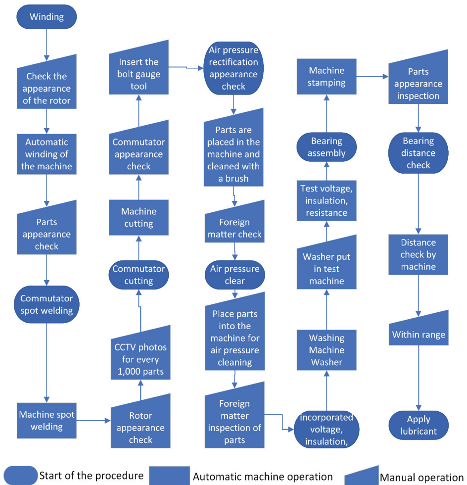
Figure 3. Coil assembly line.
