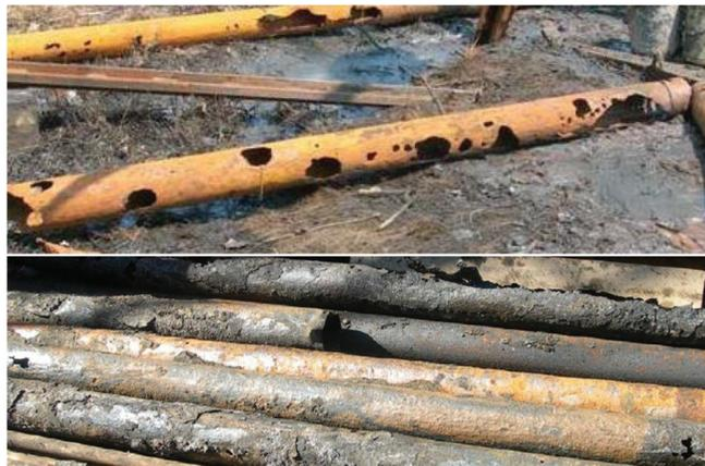
Figure 3. External steel casing corrosion from acidic water attack [32].
