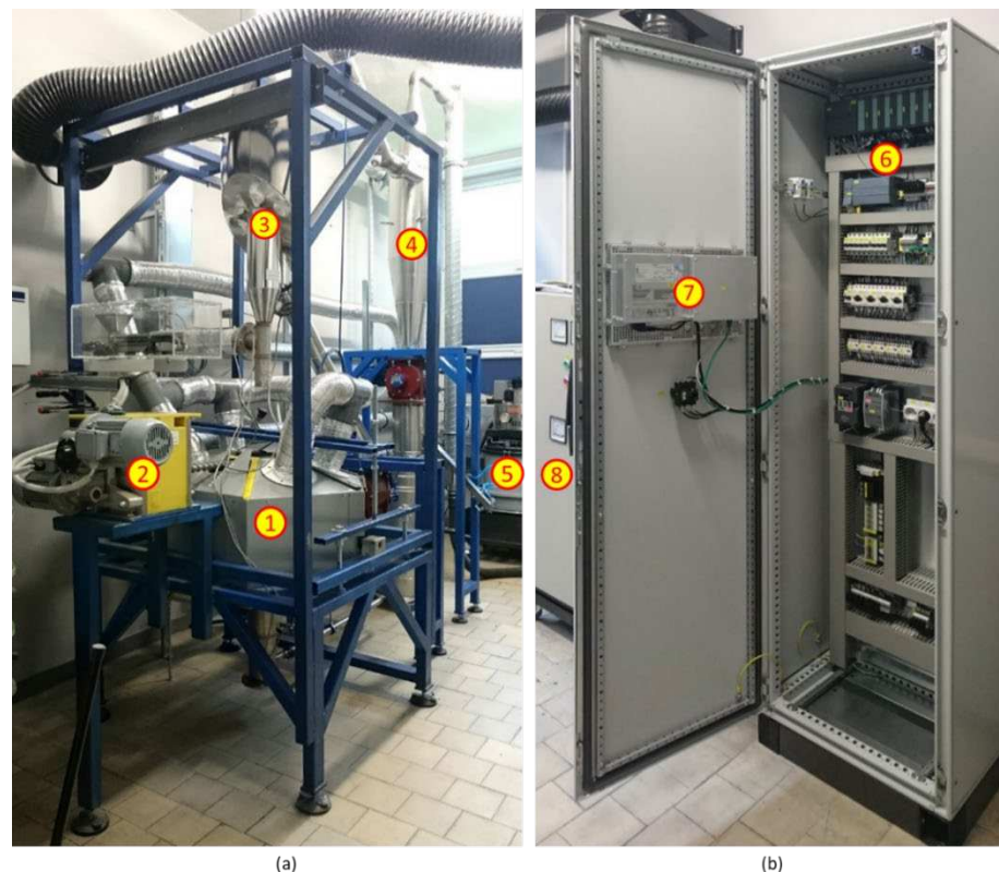
Figure 2. Semi-industrial dry grinding and classification circuit with EMM D100: (a) installation with air transport and heat recovery systems; (b) control and power supply cabinets.
