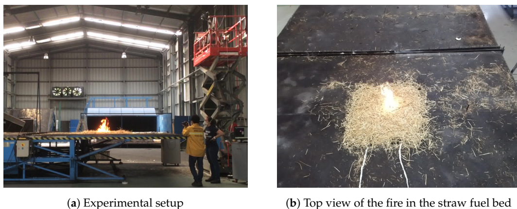
Figure 11. Laboratory trials with the FLIR SC660 mounted on an elevated platform.
