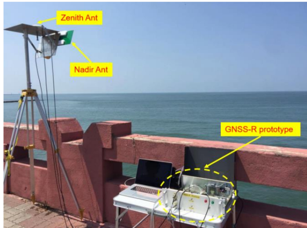
Figure 9. Ground test with the GNSS-R prototype.
