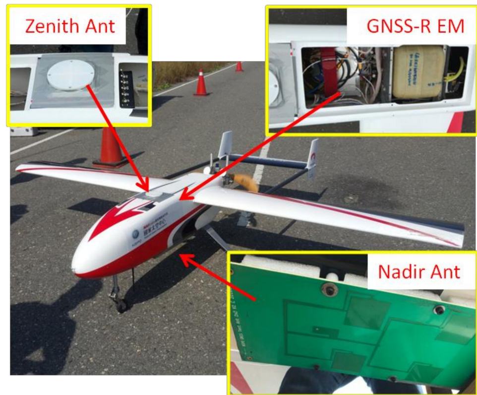
Figure 11. A unmanned aerial vehicle (UAV) flight test with GNSS-R EM.
