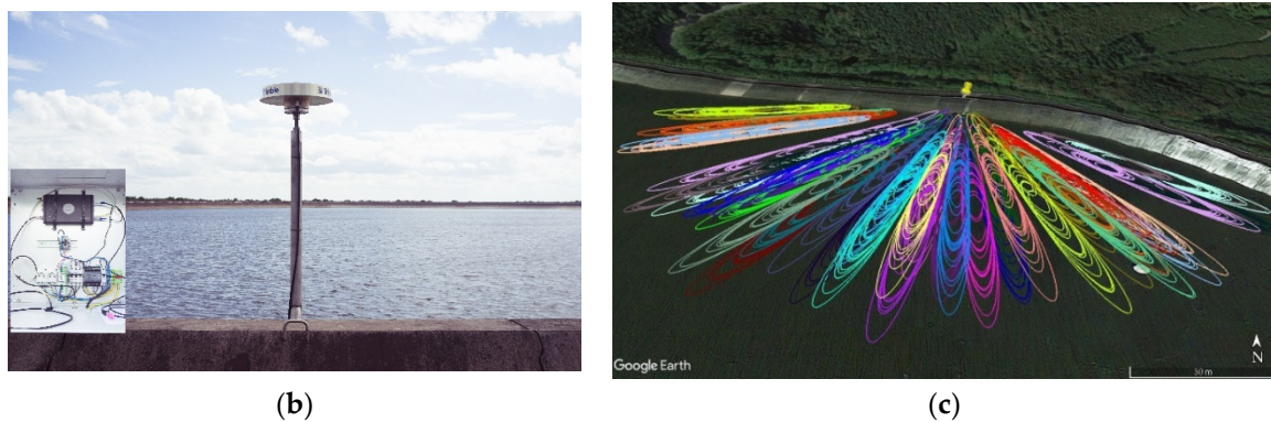
Figure 1. Vianden-pumped storage plant (a) (courtesy of the SEO, [20]), global navigation satellite system (GNSS) station VPSP at the Vianden pumped storage plant (b), and (c) occurrences of GS1C first Fresnel zones (FFZs) of July 2018 at the VPSP. Each color depicts each GPS satellite, and the location of the GNSS station is shown as a yellow pin.
