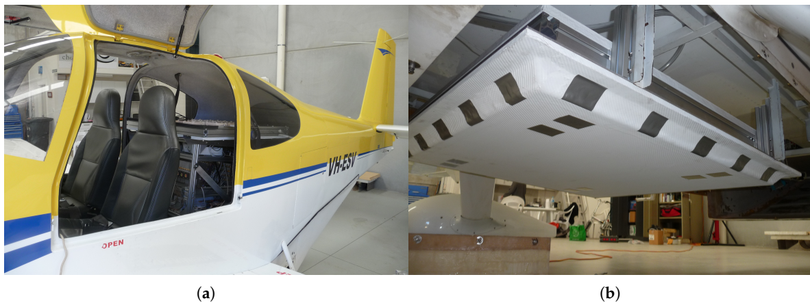
Figure 1. (a) Microwave Interferometric Reflectometer (MIR) instrument and up-looking array mounted inside the airplane, and (b) down-looking array covered with a radome hanging from the airplane's fuselage [2].
