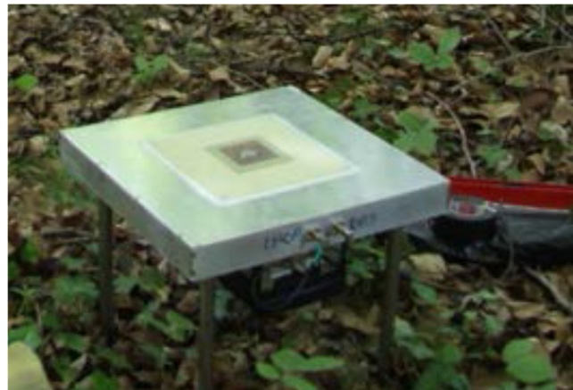
Figure 3. Dual-polarization up-looking antenna and receiver (behind the antenna) installed at La Fageda d’en Jordà (Girona, Spain).
