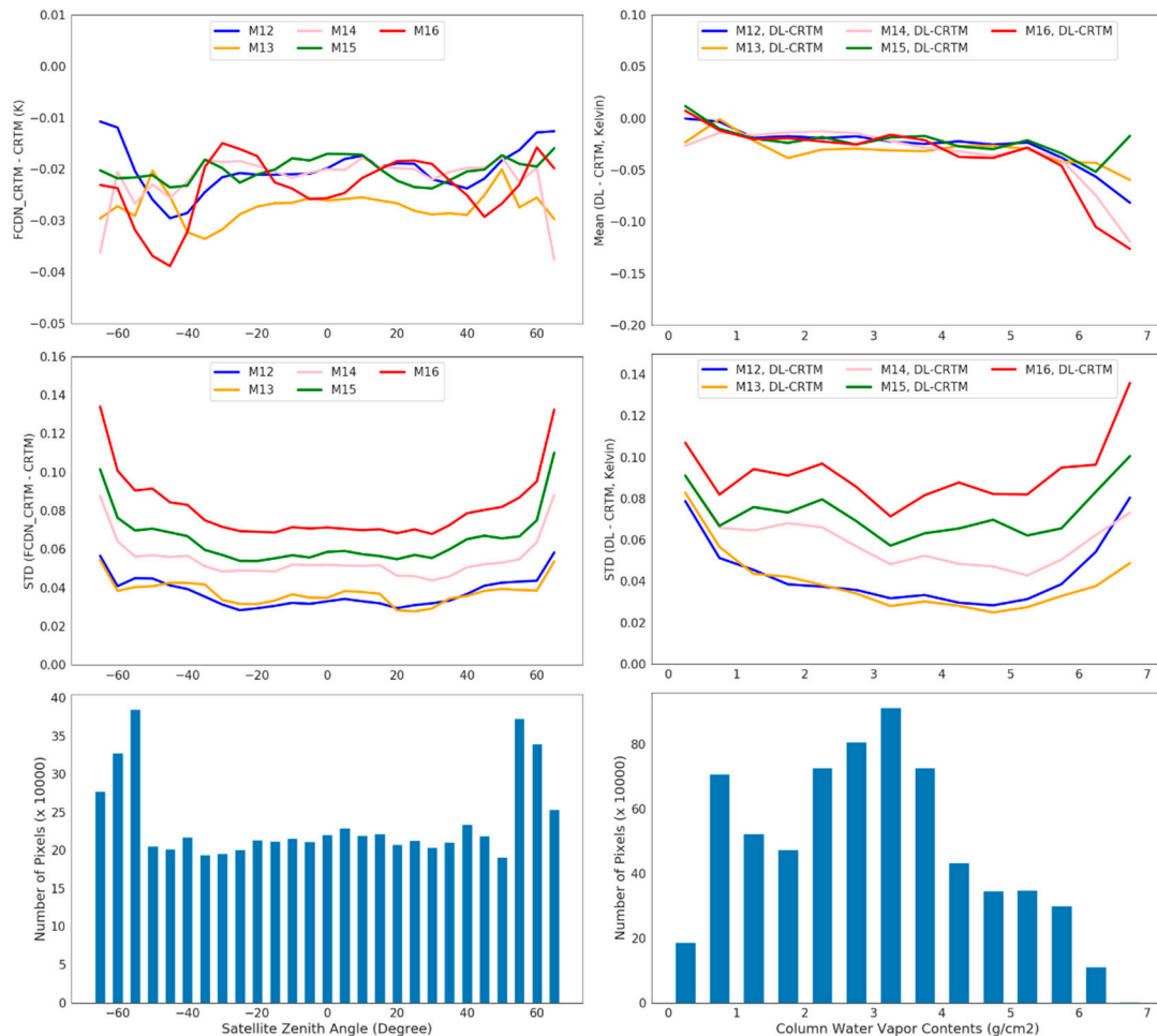
Figure 5. The F-C biases as functions of satellite zenith angle (left panel) and column water vapor (right panel) in VIIRS M12-M16 for 02/21/2020. (upper panel) F-C mean; (middle panel) STD; and (bottom panel) corresponding histogram.
