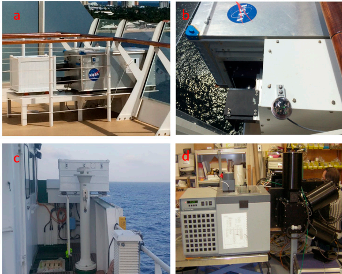
Figure 1. Installations of Marine-Atmosphere Emitted Radiance Interferometers (M-AERIs) on cruise ships (a,b). The instruments are inside hermetically sealed aluminum enclosures, with the fore optics on the aft, sheltered sides of the enclosures. The smaller boxes contain air-conditioning units to limit temperature and humidity variations in the instrument enclosures. (c): An M-AERI installed on the bridge wing of the R/V Alliance. (d): The M-AERI is calibrated in the laboratory before and after each deployment using an external validation procedure.
