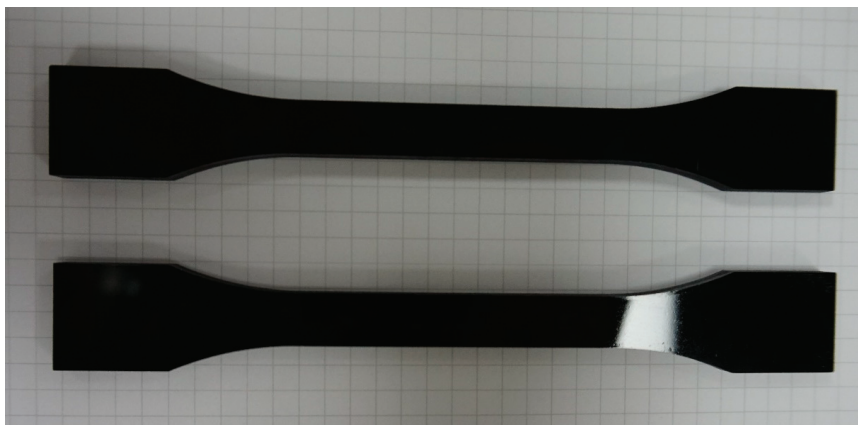
Figure 3. Photographs of moldings for tensile property testing.
