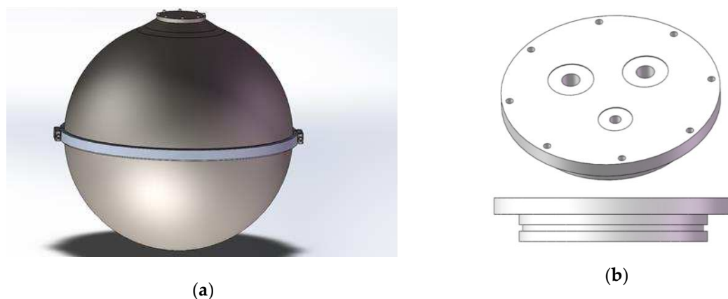
Figure 1. Sketch of the adjustable ballast tank and its sealing cover: (a) front view of the adjustable ballast tank; (b) description of the sealing cover.
