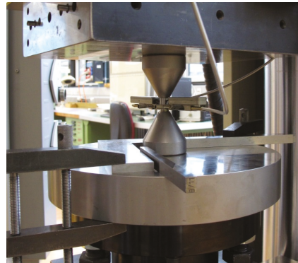
Figure 1. Schematic view of the mechanical setup (left) and installation with prepared sample in the test machine (right), with large plates adjusted and fixed in parallel.
