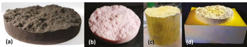
Figure 2. Preparation procedure of joint specimens; (a) 3DP mold, (b) silicone mold, (c) plaster rough joint, (d) encapsulated joint.
