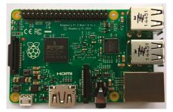
Figure 1. Raspberry Pi 2 Model B.
