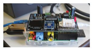
Figure 2. Raspberry Pi Model B with AirPi attached on top.
