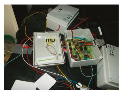
Figure 4 shows the conditioning circuit housed in a watertight box.
