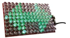
Figure 6. Double arrow shown on the LED-matrix display.
