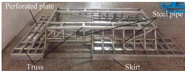
Figure 1. Photograph of the physical model.
