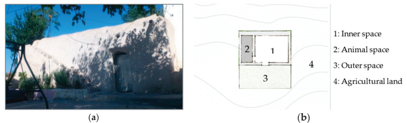
Figure 1. A traditional residential unit in the first phase, Jableh countryside. (a) The house; (b) the layout (source: photo and figure by N. Khadour).
