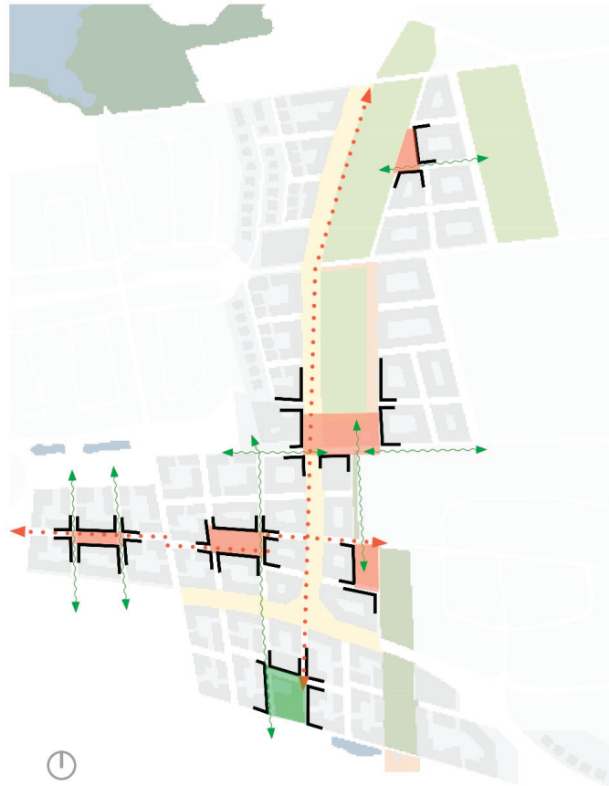
Figure 12. The concept of the new neighborhood squares is based on the networking of the neighborhood squares in the direction of N-S and W-E. A sequence of a Park-Plaza-Open space is supported by the networking of the open spaces (different types of program). Diagram, without a scale. Own elaboration based on the digital ALKIS Stadtgrundkarte (2018) of the city of Wolfsburg.
