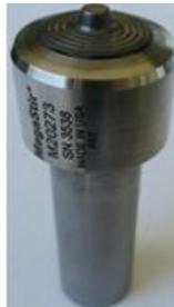
**Figure 3.** Megastir Q70 (PCBN/WRe) tool.
