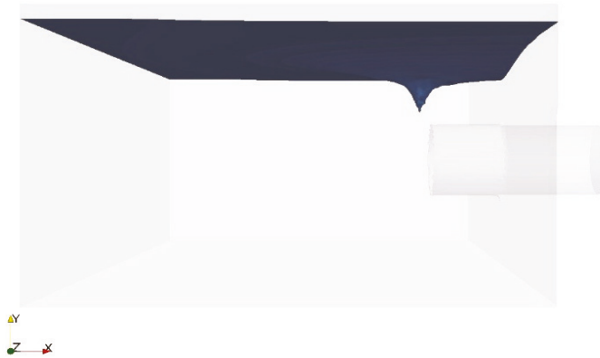
Figure 3. Vortex formed at the intake (side view).
