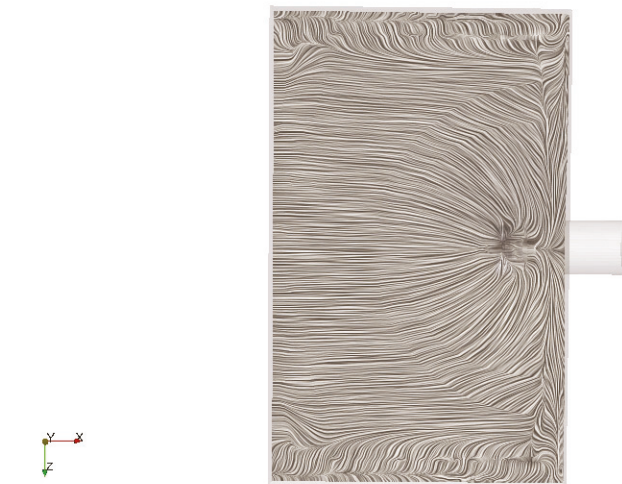
Figure 4. Streamlines illustrated with surface line integral convolution.
