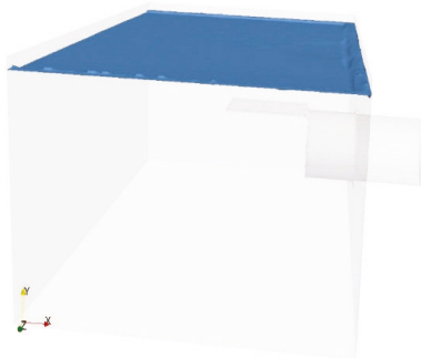
Figure 8. A slight surface depression formed in the presence of the anti-vortex plate.
