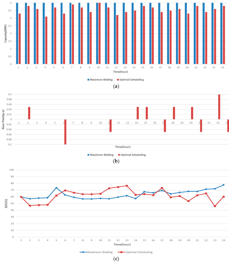
Figure 3. Maximum capacity bidding plan and optimal scheduling algorithm results (a) bidding capacity; (b) base point; and (c) SOC.
