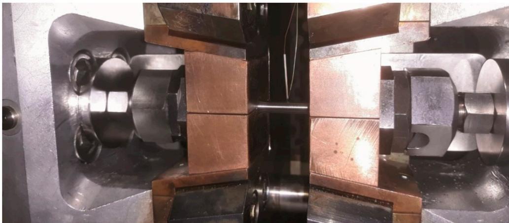
**Figure 12.** Position of sample in the Gleeble 3500 device before the temperature cycle application.
