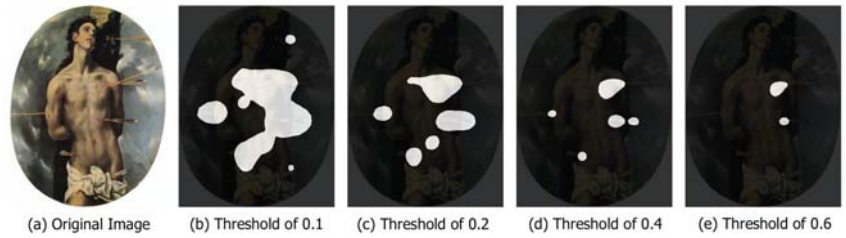
Figure 5. Analysis with different thresholds—black areas correspond to class activation map values below the specified threshold (background) while white pixels correspond to class activation map values greater or equal than the threshold (foreground). An increment in the threshold value results in smaller and more distinct areas. Original image (a), cam with threshold at 0.1 (b), cam with threshold at 0.2 (c), cam with threshold at 0.4 (d), cam with threshold at 0.6 (e).
