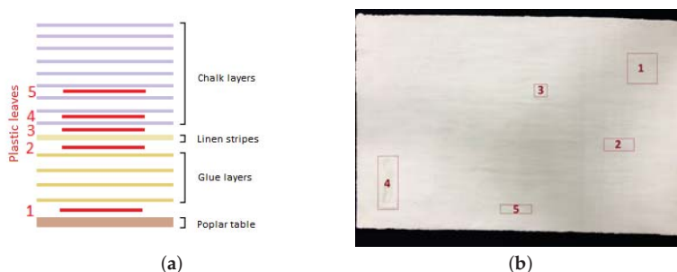
Figure A1. The fabricated painting model (40 × 60 cm): (a) scheme of the layered structure with the defects; and (b) picture with the position of the defective regions (numbered in red boxes).
