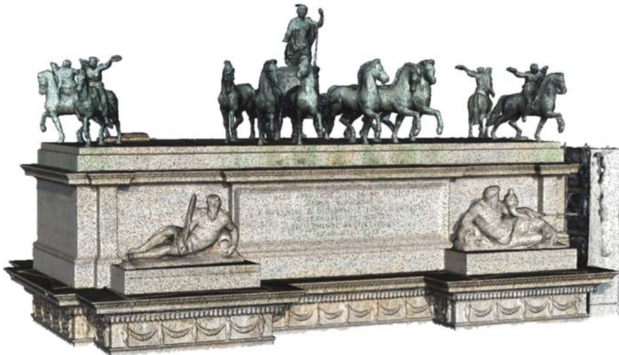
Figure 10. UAV photogrammetric dense cloud of the upper part of the arch.
