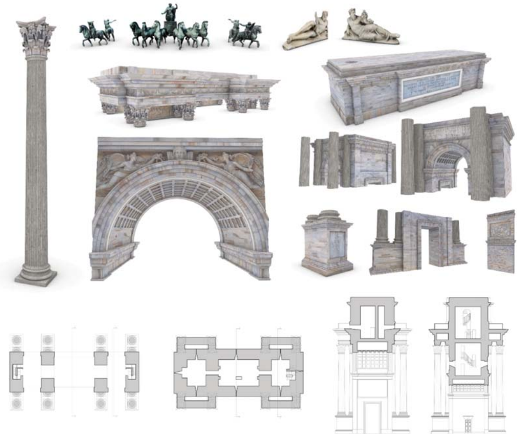
Figure 15. The HBIM objects of the research case study and the main 2D drawings extracted from the HBIM project browser.
