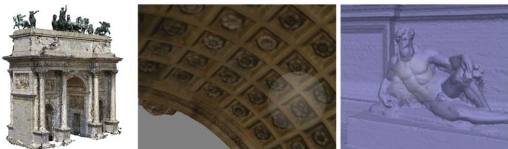
Figure 13. On the left, final merged 3D point cloud. In the centre, decorative apparatus recorded from the terrestrial photogrammetric survey; on the right, 3D model of one of the statues on the top of the arch acquired with the UAV survey.
