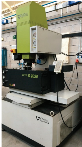
Figure 3. Electrical discharge machining (EDM) machine ONA Datic D-2030-S.
