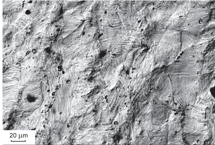
**Figure 6.** Deformation-induced surface microrelief after torsion at 299 K of coarse-grained specimen of  $\text{Ti}_{49.3}\text{Ni}_{50.7}$  (at%) alloy (details in text). Scanning electronic microscopy.
