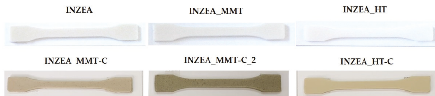
Figure 5. INZEA-based bionanocomposites containing unmodified nanoclays and chlorophyll hybrid nanopigments at 7 wt%.
