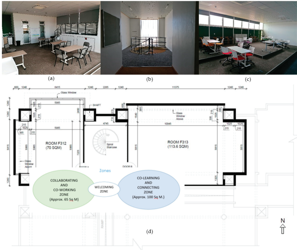
Figure 4. Case 2 working area divided into several zones with different activities. (a) Collaborating and Co-working zone; (b) Welcoming zone; (c) Co-learning and connecting zone; (d) floorplan in the starting point, where the unit of length is in millimeters.
