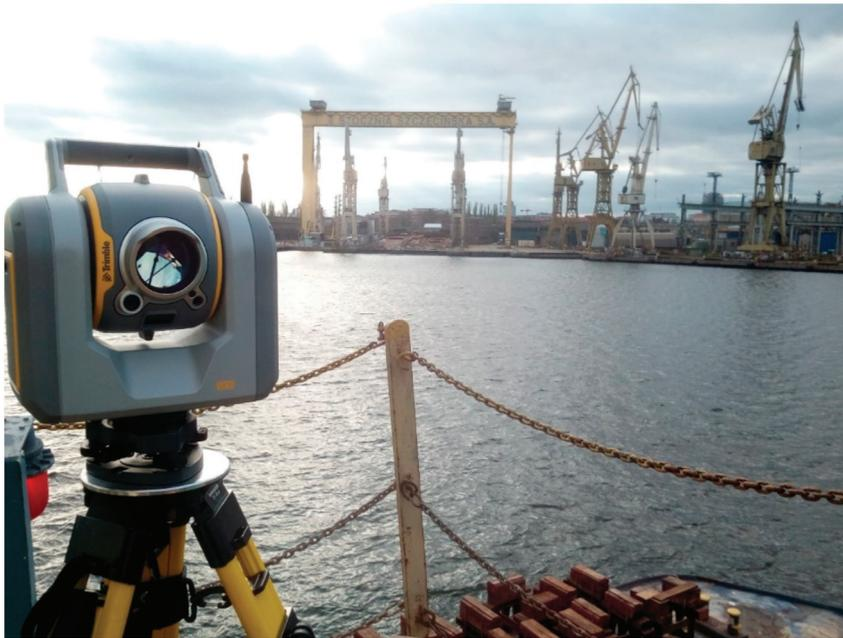
**Figure 7.** Total station measurements on a tilted reference frame (on the ship in the water).
